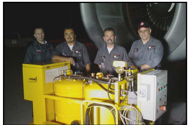
This engine-washing machine improves fuel efficiency. (Photo courtesy of Jim Walsh)
