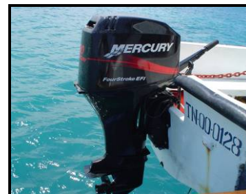
Four-stroke engine (Photo courtesy of Ecoventura)
